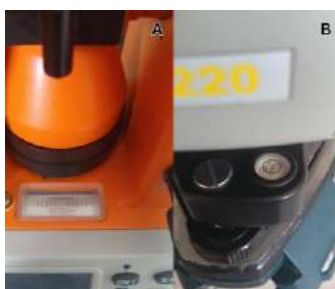
Figure 4 - The horizontal leveling (A) and the vertical leveling (B) of the theodolite.
